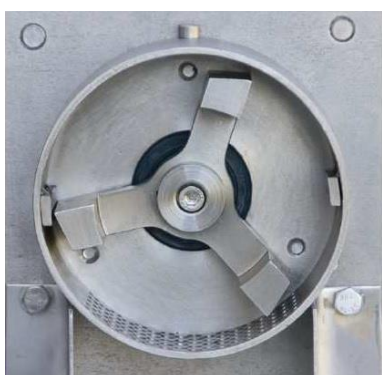
Figure 64. Internal view of olive crusher
