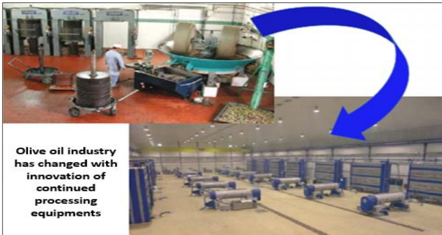
Figure 59. Olive oil production facility operating in batch and continuous system (modified from Clodoveo & Amirante, 2017)
