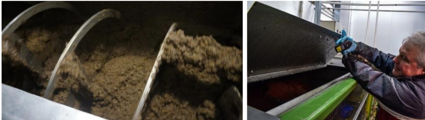
Figure 66. Internal view of malaxer and temperature measurement (batch system)
