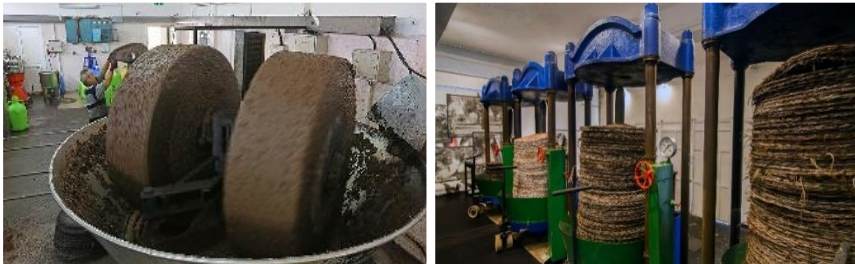
Figure 58. Photos of olive oil production in batch system (with press) (Dawson, 2020; Orfion, 2017)
